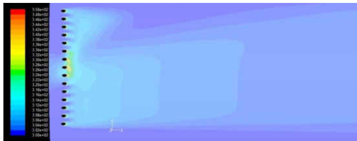
Figure 5.5: Temperature Contour of Case BR 1 Sr 0.1 at TS = 145, Spoke Location = 16.4°
