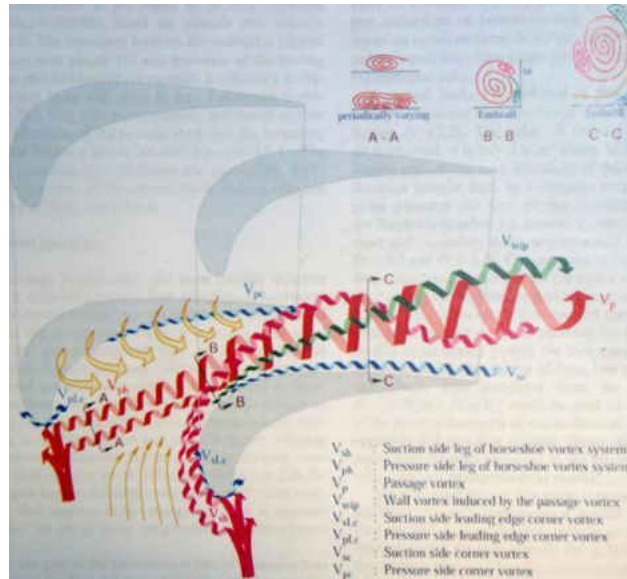
Figure 1.9: Vortexes from Rotor Stator Interaction (Goldstein and Eckerd, 1997)
